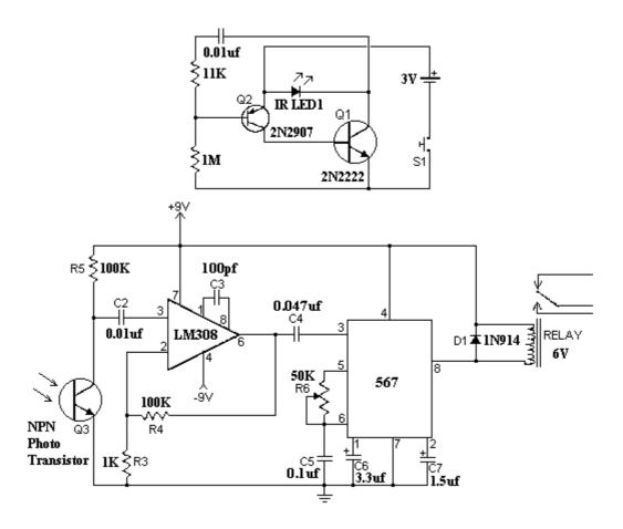
This circuits consist of two parts, the first part will transmit a signal, and the second part will detect that signal and trigger a relay. To adjust the circuit, hold down S1 while pointing LED1 at the receiver. Adjust R6 until you hear the relay click. You can increase range by using a high output LED for LED1. Bright light will stop the receiver from responding to the transmitter.
